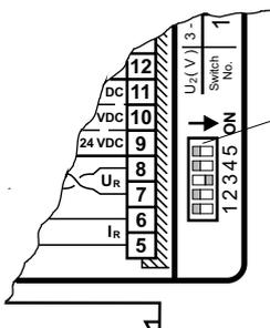
Set the DIP switch to select the secondary voltage range that will be used. With extreme low resistance heatseal elements (less than 100 mOhm) or with extremely high secondary currents (larger than 80 A) additional switch No.5 must be ON.
