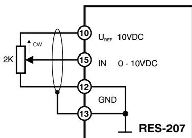
In cases when there is no analog voltage available, the temperature can be preset with an external potentiometer (2kOhm). Terminal 10 is used as the reference voltage of 10V. The digital potentiometer, P3D (P5D) offered as an accessory, is of great value since the selected preset temperature, is visible in °C in the dial window.
